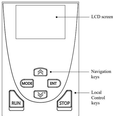
Figure 4.1 Human-Machine Interface (HMI) Front View
