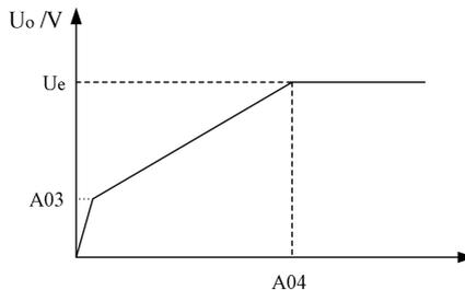
Figure 5.1 Voltage ramp
