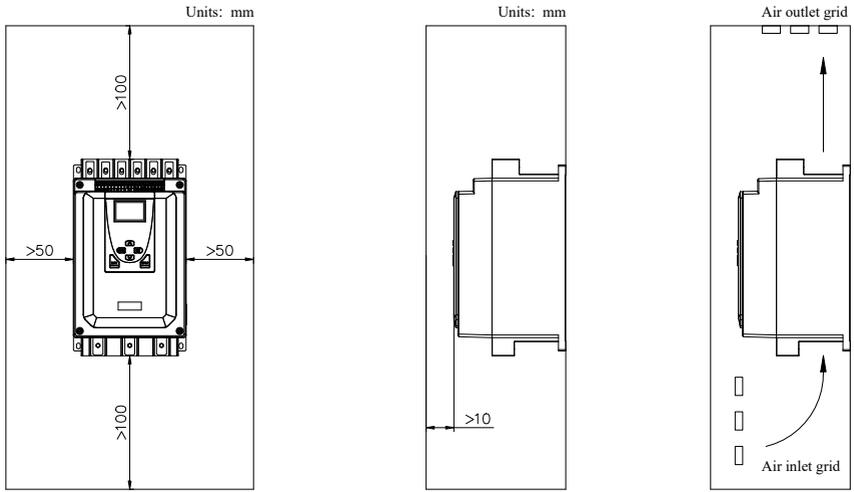
Figure 3.1 Mounting clearances
