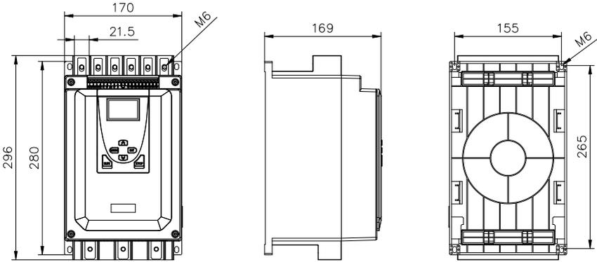
Figure 2.3 5kW~75kW (Units:mm)
